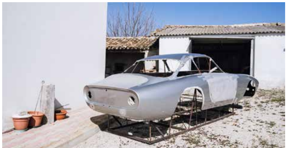
Car body in aluminium, made in 1968 by the Mario Allegretti Coachbuilders
